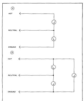
fig. 1. An illustration of the two modes of voltage transient which are encountered on a typical 3 wire circuit. (A), the case when the potential between hot and neutral is abnormally high due to a transient. (B), an alternate transient mode where the power-carrying lines are elevated above the safety ground.
